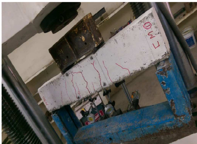
Fig-2 Failure Pattern in Beam
